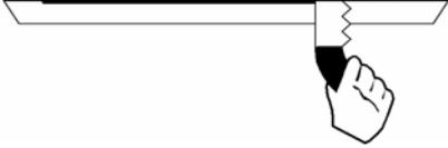
3. Fit the grille on either side of the door. At this point, building grade adhesive can be used on the inside of the flange of both grilles for a more permanent fixing. Apply around the entire perimeter.
