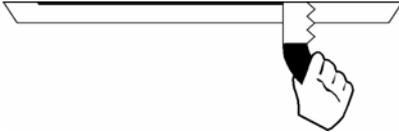
3. Pull the duct through the opening in the ceiling and attach the boot to the duct using duct tape. Or for accessible ceiling spaces duct can be attached whilst in the ceiling space once the boot is secured in place.
